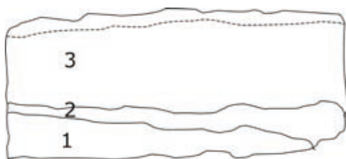
Fig. 3.A.2 Schematic layer build-up of the whitened sample (A). (1) ground layer (50 \mu\text{m} ). (2) light-brown underpaint layer (10-30 \mu\text{m} ). (3) bone black layer (80-140 \mu\text{m} ), the dashed line indicates the white top layer (10-20 \mu\text{m} ).
