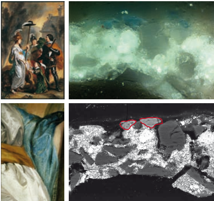
Fig. 2.26 Gonzales Coques, Frederik Hendrik Receiving Survivance for Willem II , c. 1650, Oranjezaal No. 19. Strawn azurite is used in the blue sash of Hollandia (woman at the left) to preserve the blue color ( lower left ). The SEM backscatter image of the cross-section shows that the azurite particles (outlined in red) at the surface are embedded in the smalt layer below ( lower right ). Photo (painting): Royal Collections. Photo (detail): SRAL.
