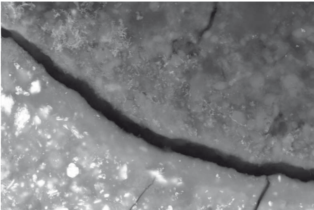
Fig. 4.5.4 SEM backscatter image showing interface between upper lead white ground and dark paint.
